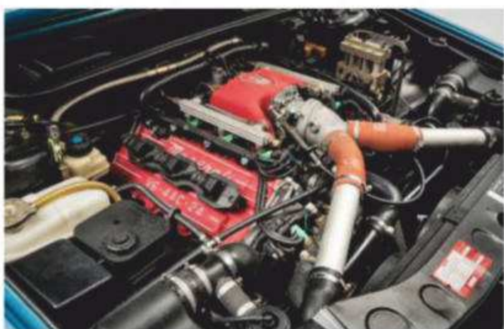
Ghibli was fitted with a twin-turbo V6 and was a development of the Biturbo. Standard UK Ghiblis came with the 284bhp 2.8-litre V6, not the 2.0-litre unit fitted to Italian-market cars
